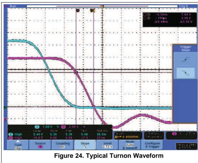
Figure 24. Typical Turnon Waveform
