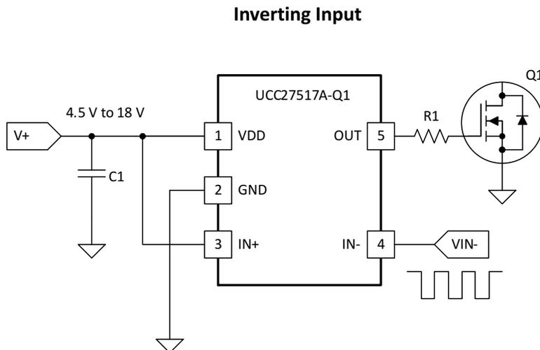
Figure 23. Using Inverting Input (IN+ is tied to V<sub>DD</sub> enable output)
