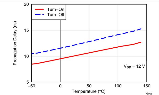
Figure 14. Input to Output Propagation Delay vs Temperature
