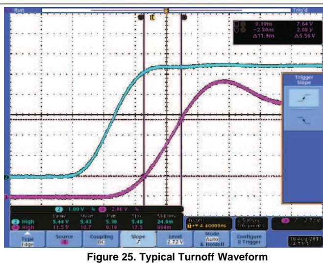
Figure 25. Typical Turnoff Waveform
